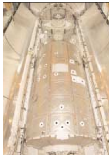
Micro-meteoroid debris shields on this NASA laboratory space module were manufactured by Superform USA.
